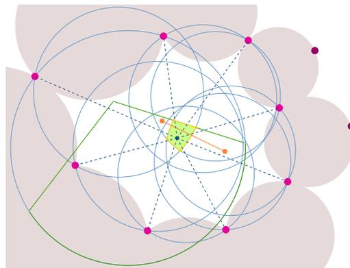
Figure 1: Sifting example (orange: candidate, purple: neighbors, green: sampling region, blue: replacement point, dashed lines: retriangulation, other: constraints).
