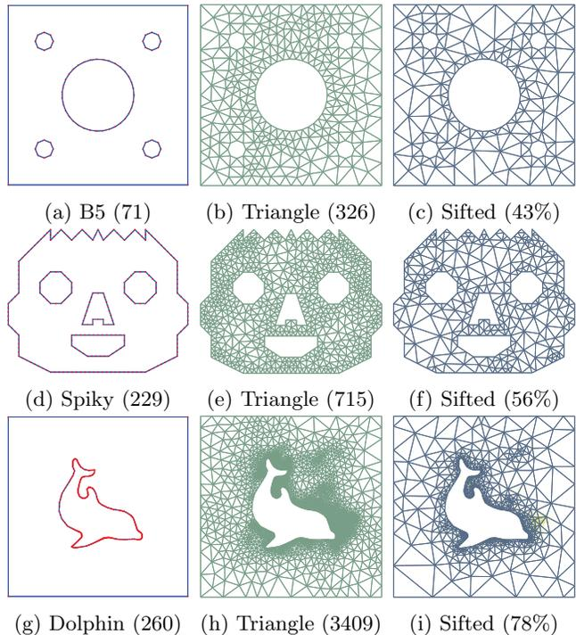
Figure 2: Model, triangle -q35 and sifted meshes.
